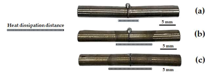
Fig. 4. The images of welded cylindrical specimens which are likely bonded using TLPB of SSM 6063 aluminum alloy with Zamak 2 binder from the bonding time of 120 min as: (a) 450, (b) 500 and (c) 550 °C.
