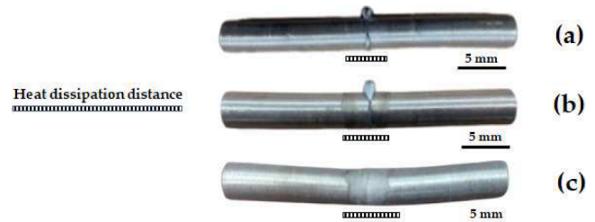
Fig. 5. The images of welded cylindrical specimens which are likely bonded using TLPB of SSM 6063 aluminum alloy with Zamak 2 binder from the bonding time of 60 min as: (a) 450, (b) 500 and (c) 550 °C.
