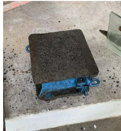
Figure 1 Preparation of sedimentary rock-based concrete blocks size 15 cm x 15 cm x 15 cm.
