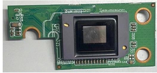
**Figure 1.** Due to a hermetic seal encompassing the DMD and its control circuits in the malfunctioning ViewSonic projector model PJD5123, we encountered difficulty in attempting to dismantle it.
