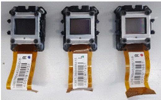
**Figure 9.** We acquired three HTPS TFT-LCDs, each accompanied by a corresponding contact block adapter, from dismantling one 3LCD technology projector.
