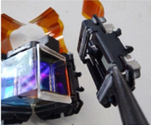
**Figure 8.** Used pliers to carefully extract the LCD contact block adapter from the dichroic prism, to which it was adhered with glue.
