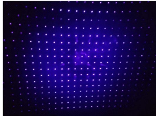
**Figure 14.** The diffraction patterns generated by the blue laser ( $405 \pm 10$  nm) were projected onto the dark-room wall.
