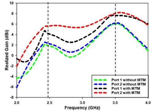
Figure 4. Realized gain of the proposed antenna and two-port MIMO antenna without MTM.
