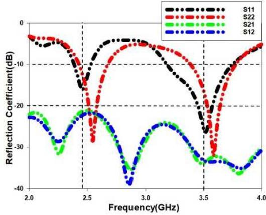
Figure 3. Simulated results for gap of  $0.1\lambda_{guided}$  S11, S22, S21 and S12.
