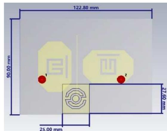
Figure 1. Proposed MIMO MTM textile antenna.
