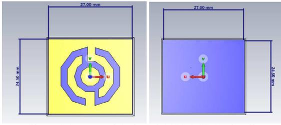
Figure 2. Decagonal C-shaped CSRR MTM unit cell.
