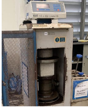
Figure 2 Assessment of Compressive Strength
