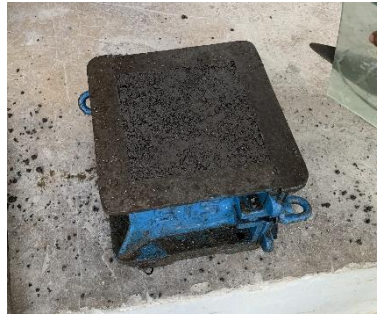
Figure 1 Preparation of sedimentary rock blocks of size 15 cm x15 cm x15 cm
