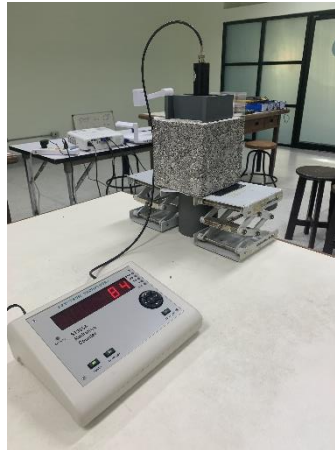
Figure 3 Examination of the radiation shielding characteristics of sedimentary rock block bricks
