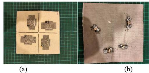
Fig. 6. Photograph of the fabricated MIMO textile antenna (a) Front view and (b) back view.
