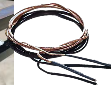
(ก-9) Thermocouple Type K
