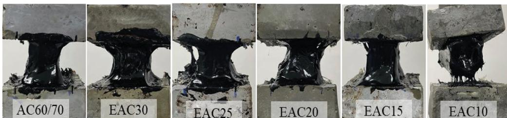
**Figure 8.** Failure images for bonding between modified epoxy asphalt products and concrete.
